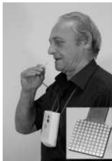
Fig. 1. The BrainPort Balance Device. Electrode Array.
